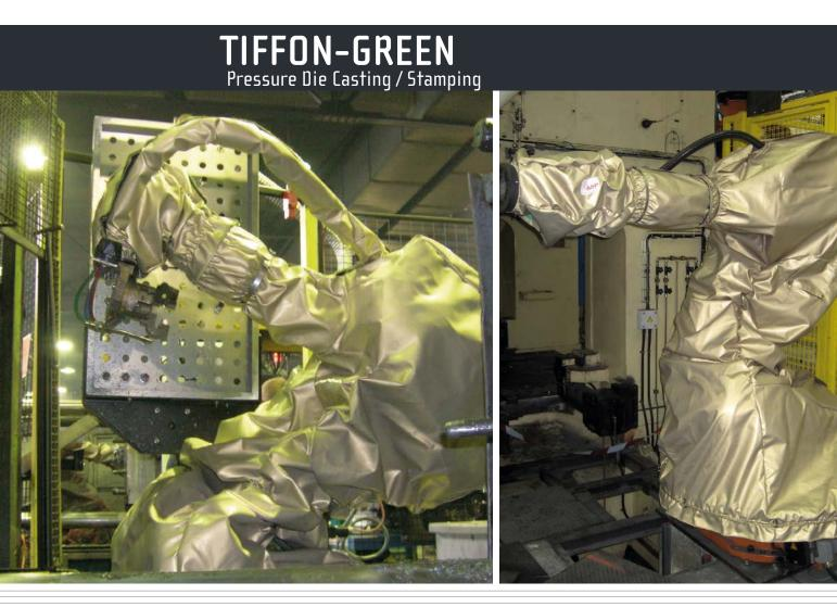
High tearing strength M1 class flameproofed fabric Stands up to aluminium, brass,
