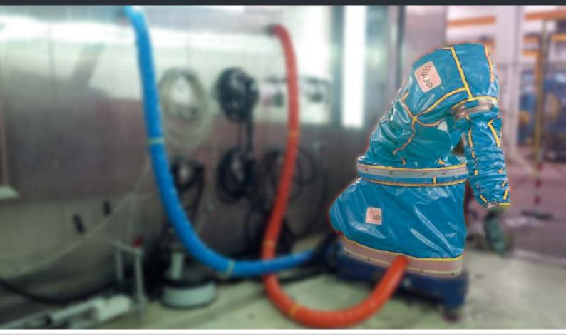
Multiple-layer insulating cover to impede heat transfer
