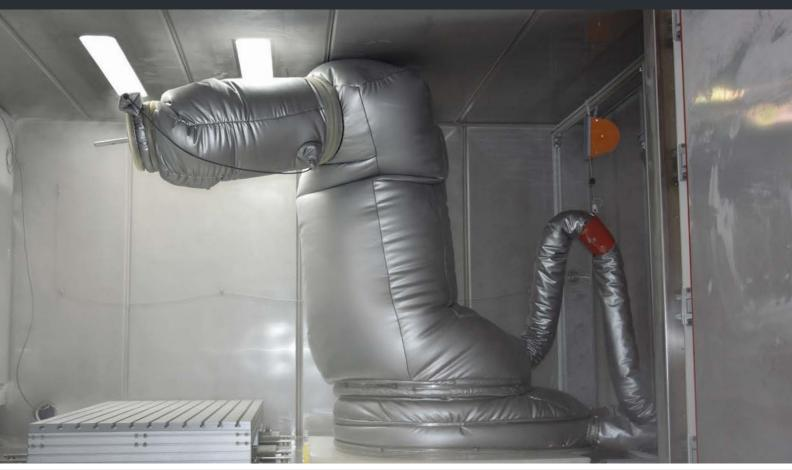
Multiple-layer insulating cover to impede heat transfer
